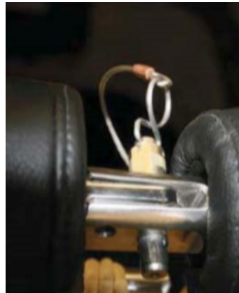
Top Bar in closed position with release pin installed
