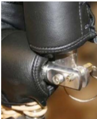
Top Bar raised with stopping pin installed
