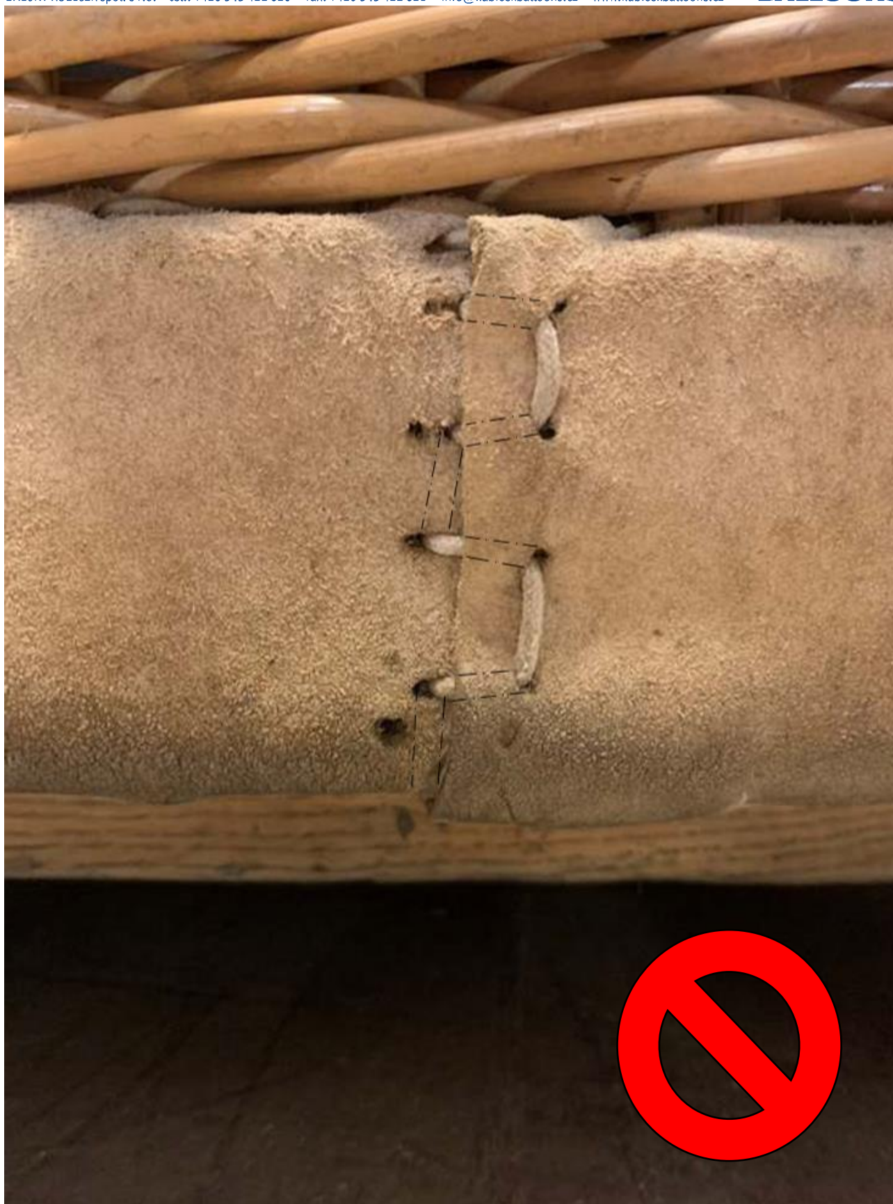
Fig. 11: Connection of two rawhide leathers together (please note, that in picture is used basket and it only represents method of connection, however on new product are holes in both pieces at same line – see Fig. 10). This offset happens, when connected leathers are still wet, because during drying leather is shriveling.
