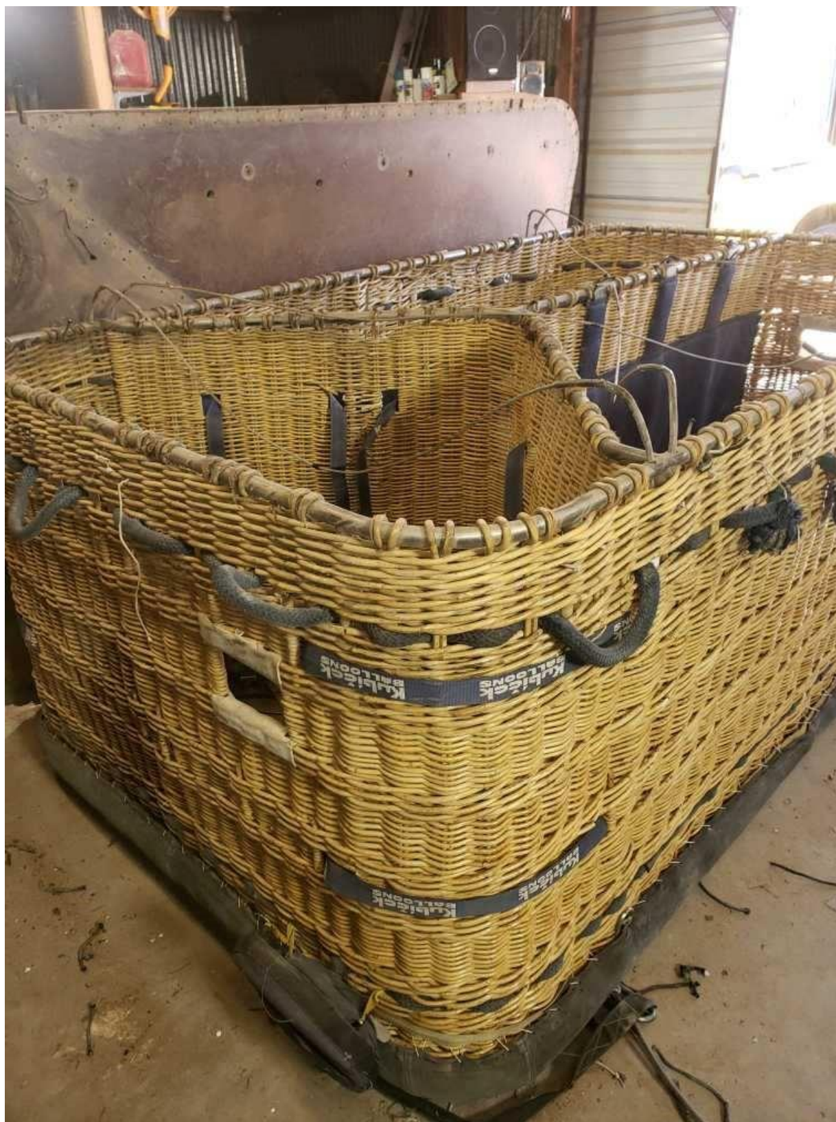
Fig. 3: Condition of rest of basket after floor disassembly
