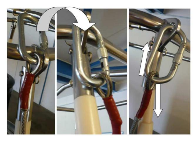
In order to prevent this issue we highly reccomend installation of "Basket wire stopper", order no. 54725.00. Just put on the karabiner the rubber eye as seen on the following picture.
